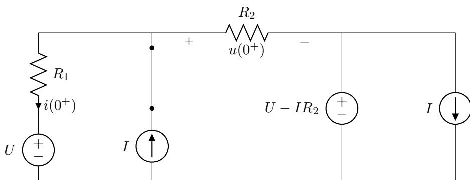
Notice that the actual current-source  $I$  (the rightmost branch) is irrelevant to the two variables we're looking for: there is a voltage-source in parallel with it ( $U - IR_2$ , the voltage on  $C_2$ ).
