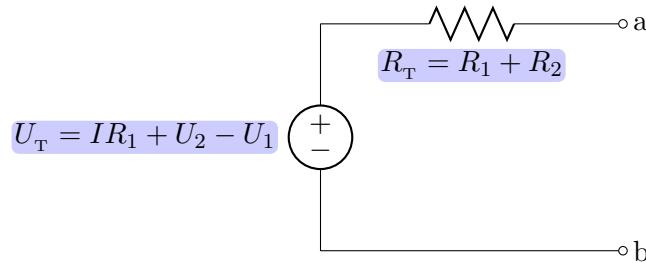
To find the open-circuit voltage (equal to Thevenin voltage) notice that if a-b are open-circuit then there is no voltage across  $R_2$ , and all the current  $I$  must pass downwards through resistor  $R_1$ ; then KVL around  $R_2$ ,  $U_1$ ,  $R_1$ ,  $U_2$  and a-b gives the open-circuit voltage  $u_{ab(oc)}$  of 'a' relative to 'b'
