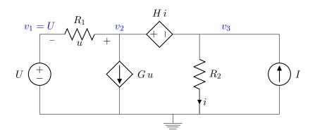
If the bottom node is the reference, then the node  $v_1$  becomes part of the 'ground supernode'; we already know its potential, and we don't need any KCL.
