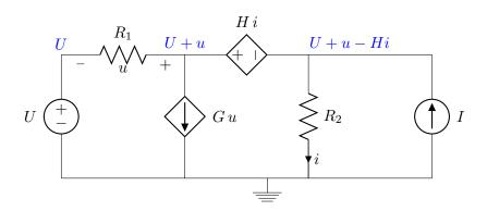
The current *i* is, by Ohm's law,  $i = \frac{U+u-Hi}{R_2}$ . Rearranging,  $i = \frac{U+u}{R_2+H}$ .
