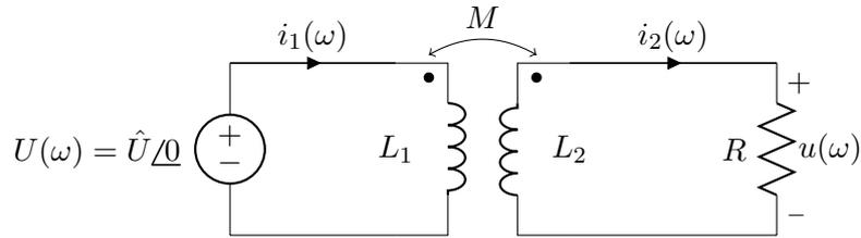
The equations for mutual inductors, and Ohm's law for the resistor, are:
