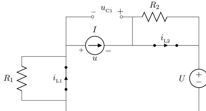
The energy stored in the capacitor is  $\frac{1}{2}C_1u_{C_1}^2$ .
