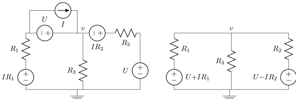
**Source transformation and simplify current-sources.** A quite similar simplification can be done using just one source transformation, if one realises that node ‘a’ in the original circuit has current sources putting equal currents in *and* out; their total current is therefore zero, so they do not affect the node. These sources can then be separated as shown below, and simplified into one.
