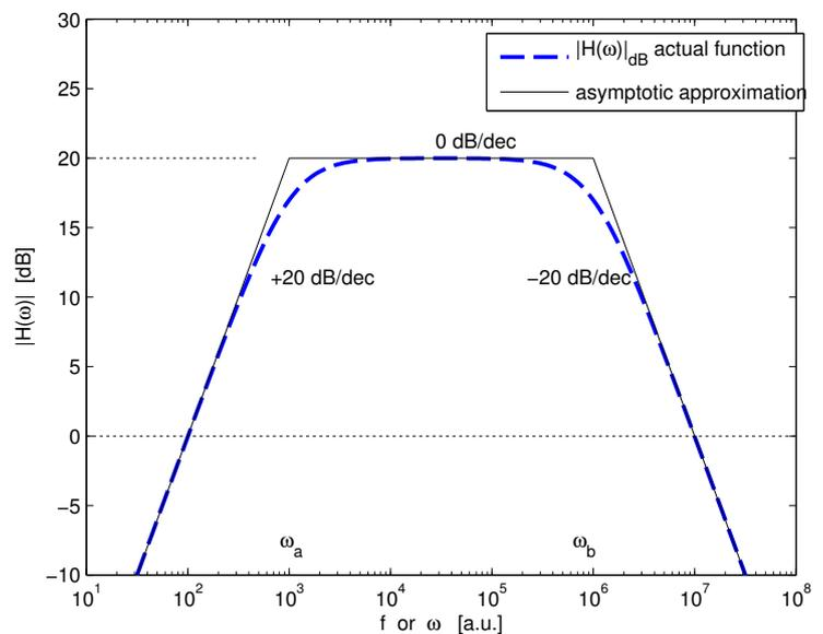
The Bode magnitude diagram can be worked out from the function itself, considering approximations when the frequency is at, or is much above or below, the special frequencies  $\omega_a$  and  $\omega_b$ .
