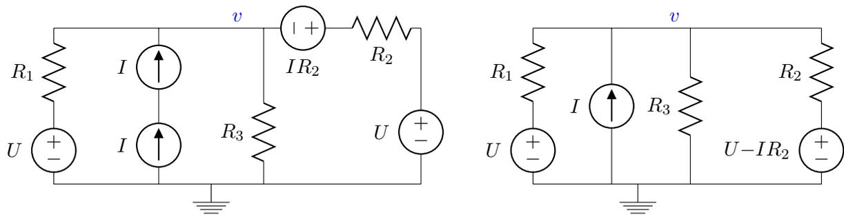
( This simplification of current sources is one of many ‘theorems’ for circuits.
