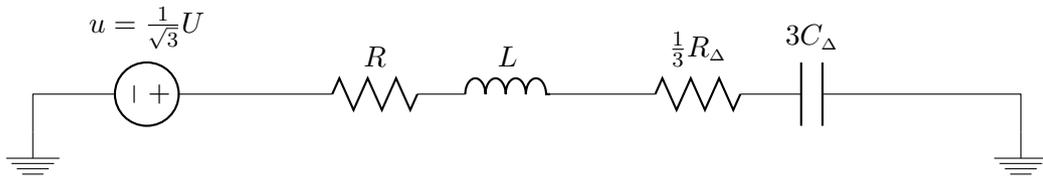
In the single-phase circuit above, the source provides a complex power of
