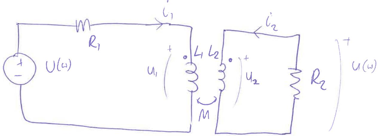
Identical to the original circuit with  $U_1, U_2, i_1, i_2$  added.
