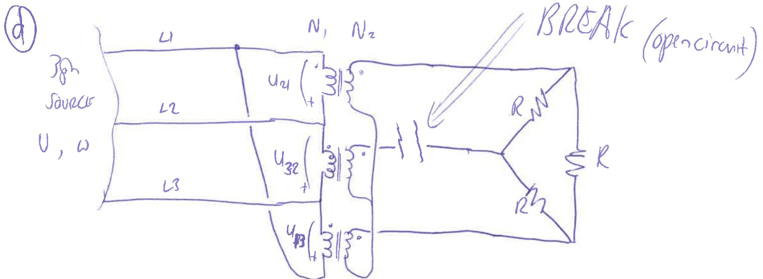
The break prevents all current in the middle transformer, since its secondary current is 0 so its primary current is also 0.
