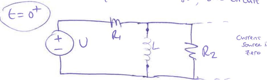
'Seen' by the inductor, the rest of the circuit is a Thevenin equivalent of:
