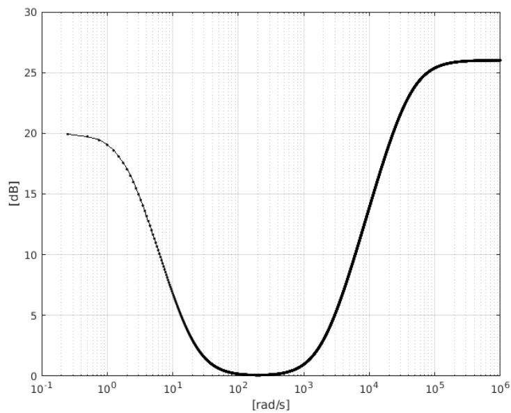
$$\rightarrow H(\omega) = \sqrt{100} \frac{(1+\frac{\omega}{20})(1+\frac{\omega}{2000})}{(1+j\frac{\omega}{2})(1+j\frac{\omega}{40000})}$$
