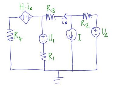
b. Using 'extended' nodal analysis (wherein no simplifications are made, but a set of equations is written based on a few simple rules), how many equations will be used to represent this circuit?
