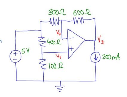
**c.**  $v_3$ KCL at  $v_2$ :  $(v_2 - 5 \text{ V}) / 300 \Omega + 0 + (v_2 - v_3) / 600 \Omega = 0$ . We already have  $v_2 = 1 \text{ V}$ , so this KCL gives a solution of  $v_3$ .  $v_3 = (-4 \text{ V} / 300 \Omega + 1 \text{ V} / 600 \Omega) \cdot 600 \Omega = -7 \text{ V}$ .
